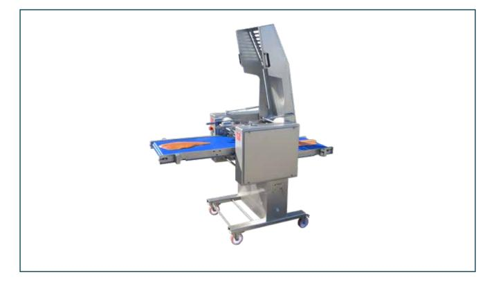
The Skinning machine V1578 is a single lane skinning machine specially designed to deep skin smoked salmon.
