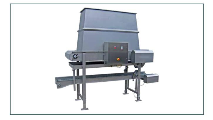
The ice doser is built for automatic filling of ice into boxes with fish.
