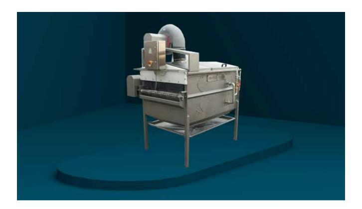
The Fillet washer 700 is a fully automatic fillet and fish washer for removal of slime and bacteria from processed fillets.
