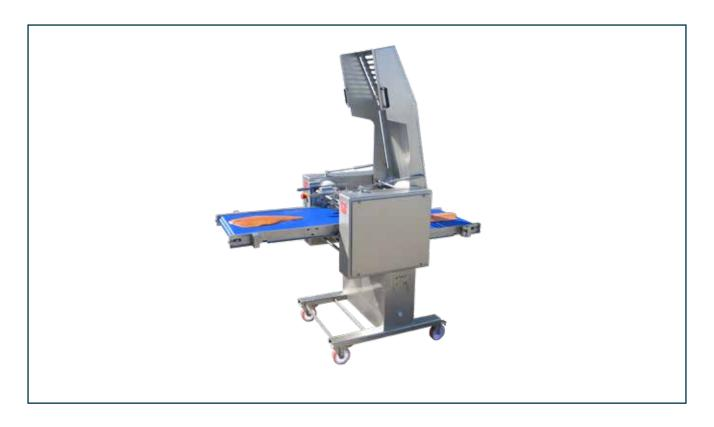
The Skinning machine V1578 is a single lane skinning machine specially designed to deep skin smoked salmon.
