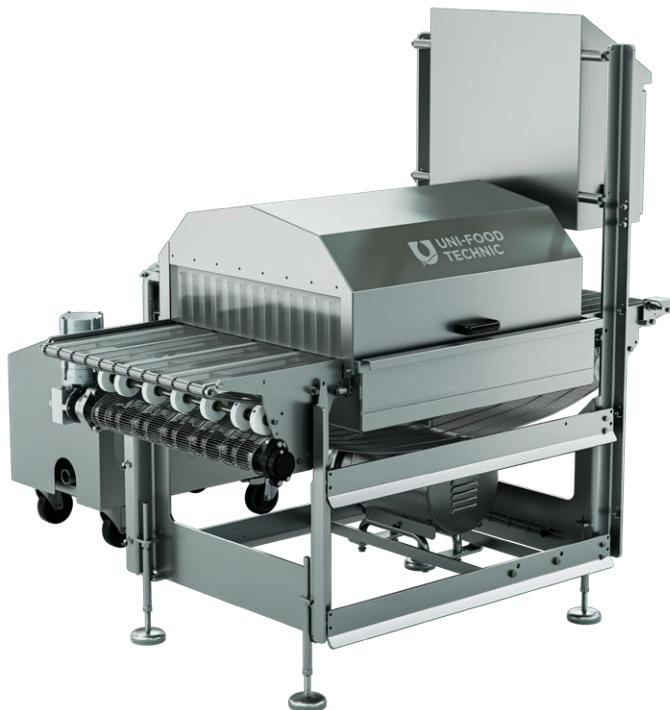
The Fillet Washer 700 is a fully automatic solution designed to remove slime and bacteria from processed fish fillets, ensuring a clean and hygienic end-product.
