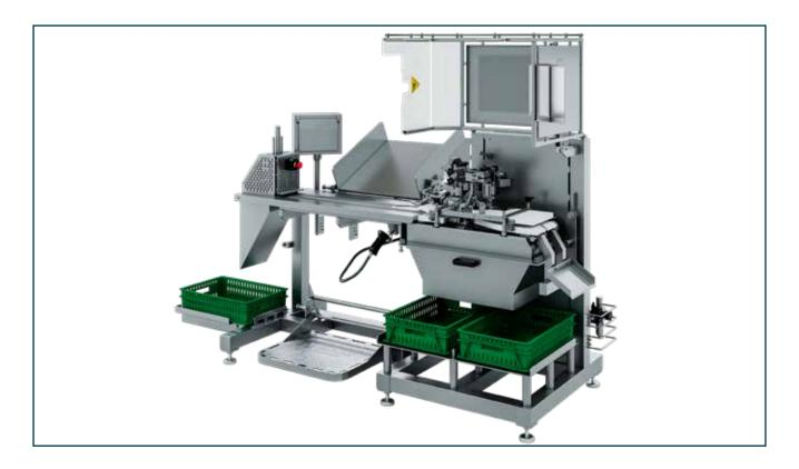
The scraping machine SP 60J is designed to scrape the remaining meat off the salmon backbones after skinning. It offers the making of a high-end by-product.
