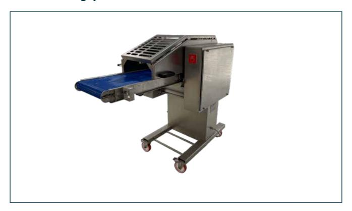
The Skinning machine V1358 is a narrow, single lane skinning machine that is designed to skin all types of fillets.
